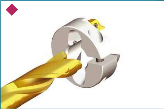
1. Insert the chamfering ring on to the drill body. The stopper must be inside the flute.
