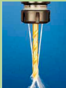
Sealed Collet Jet2 With angular double nozzles. Coolant flow is direct to the cutting edge, for use with standard straight shank cutting tools (without coolant hole).
