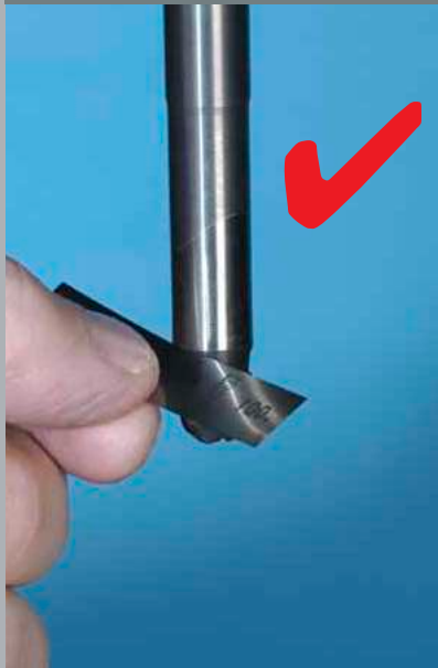
Figure 3b. Proper fit
