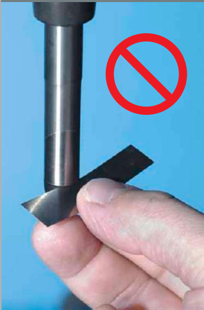
Figure 3a. Shim should NOT enter intersection
