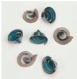
Too tight: Increase speed within recommended limit. If unsatisfactory, decrease feed.
